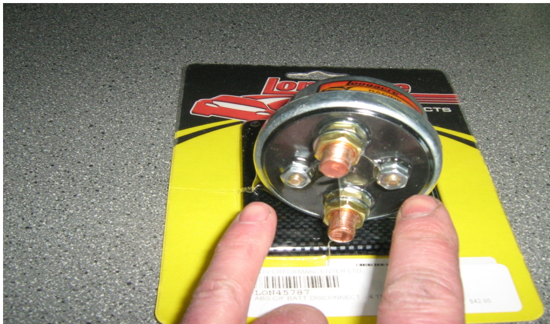
Pic 2 - Typical Kill switch with heavy terminals for battery cables and smaller terminals for alternator field disconnect.
