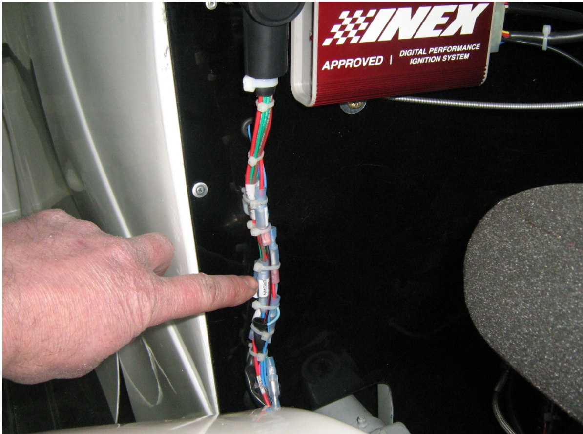
Pic 3 Alternator field wire location - factory label "ALT Brown".
